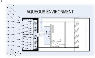
. C.L.A.M.s weigh just over one pound, including the 4 AA batteries, and many can be easily taken to remote areas and left unattended to sample continuously for up to 36 hours at submerged depths up to 100 feet in marine or fresh waters.
