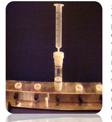
Solvent elution of the field extracted disk follows EPA method 3535 for SPE elution procedures, it simply has to be solvent eluted and concentrated to a set extract volume. The extract solvent selection is instrument dependent. Our analysis required the use of GC/FID and GC/MS/MS so acetone and DCM were the elution solvents. The elution of the disks are performed in standard vacuum manifolds or with a simple syringe forcing or drawing solvent through the SPE media.
