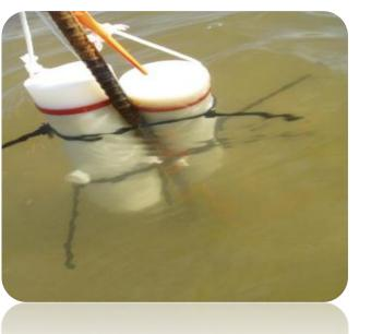
The total volume in liters extracted was calculated from this information, and was recorded on the chain of custody for the analytical quantitation. Results were reported in PPT for the PAH's due to the large volume of water usually (60-80 liters), that was extracted. The enhanced extraction volumes allowed almost two orders of magnitude lower detection, than a standard 1 liter grab sample.
