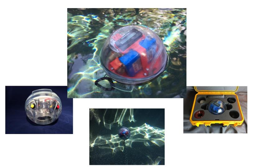
Above are photos of the Continuous Low-level Aquatic Monitoring device called the CLAM . The CLAM comes in a field ready case with accessories shown in the photos above. The CLAM should be treated as an instrument and not subjected to severe jolts or rough handling.
