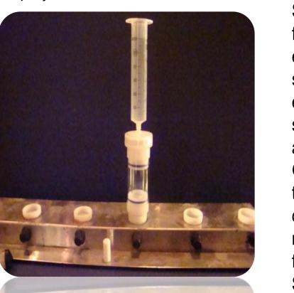
Solvent elution of the field extracted disk follows EPA method 3535 for SPE elution procedures, it simply has to be solvent eluted and concentrated to a set extract volume. The extract solvent selection is instrument dependent. Our analysis required the use of GC/FID and GC/MS/MS so acetone and DCM were the elution solvents. The elution of the disks are performed in standard vacuum manifolds or with a simple syringe forcing or drawing solvent through the SPE media.
