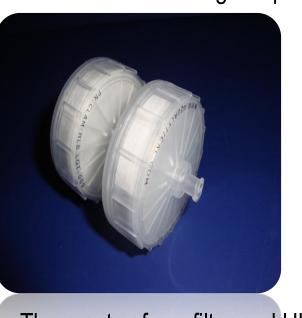
Total and dissolved organics were determined using a two stage Luer-Lok filter disk system. The first disk is a 1.5 micron depth filter disk, which removes and collects suspended trace organics, sediments and oil droplets. The second a HLB media disk which sequesters the dissolved trace organics and water oil emulsions.
