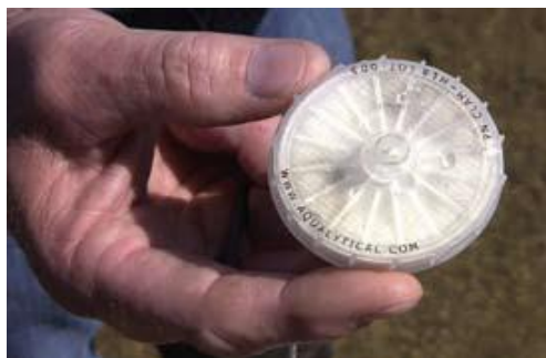
C.L.A.M. disk - that's all that gets sent to the lab, leaving the water behind
