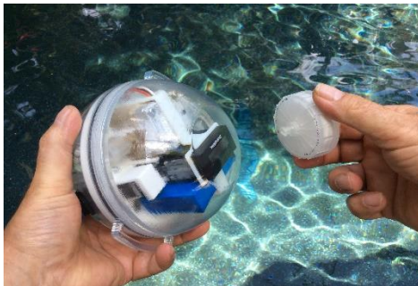
The C.L.A.M. provides a convenient submersible sealed unit with clear visual volume display, external control, and 48 hours of continuous submersible operation.
