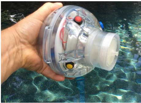
C.L.A.M. with onboard totalizer and external digital display reset and pump control buttons.
