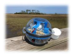
The extraction event is powered by a small subersible pump. It draws the water through the disks while floating or submerged at flow rates of 50-70 ml/min. The lofted pre-filtration and the gentle flow rates allow for the extraction of up to 100 liters in most fresh or marine waters, and can operate for 36 hours, using a rechargable lithum ion battery
