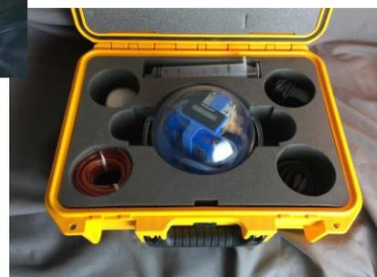
Above are photos of the Continuous Low-level Aquatic Monitoring device called the CLAM . The CLAM comes in a field ready case with accessories shown in the photos above. The CLAM should be treated as an instrument and not subjected to severe jolts or rough handling.
