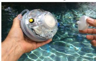
Disks if being used in a 2 or 3 stage deployment (a pre-filter disk can be used in front of a media disk for total and dissolved studies), ensure that the CLAM is just about ready to be put in the water.
